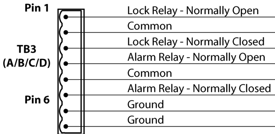
Figure 13: A-Door Lock Relay and Alarm Relay Connections (TB3)
