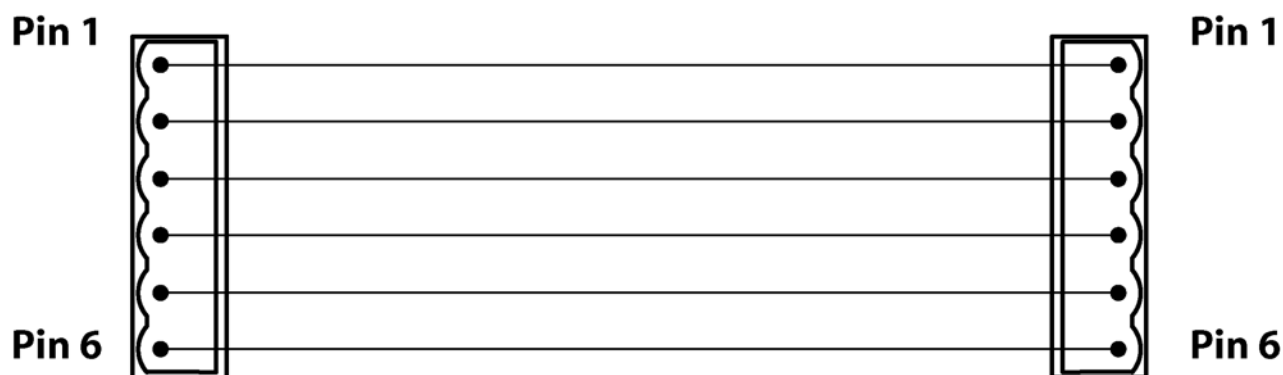
Figure 29: TB10 Jumper Cable Wiring
