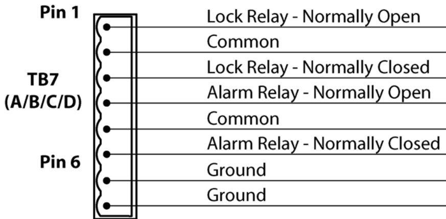
Figure 14: B-Door Lock Relay and Alarm Relay Connections
