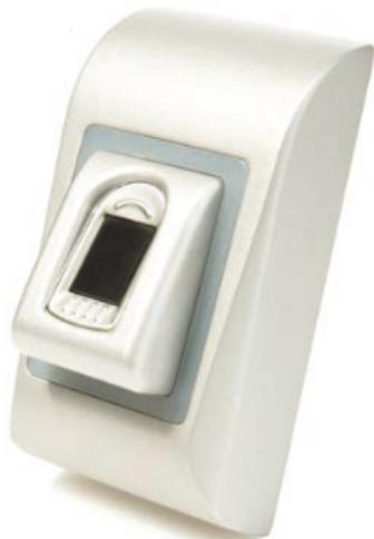
The KBF-1FP is a Wiegand biometric reader for indoor access control applications. It offers storage of up to 9,500 fingerprints and has programmable Wiegand output (8 to 128 bits). Configuration of the readers and the users is performed using the BioManager software and is covered further on in this section. Connection between biometric readers is via an RS-485 network. This RS-485 network is also used for fingerprint transfer and unit configuration.
