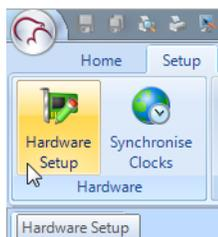
Hardware setup has six tabs; Doors, Inputs, Outputs, Panels, Cameras, and All. When you highlight an item in any of the trees under a tab the associated properties will appear in the grid on the right. Note that some hardware properties are only visible when 'Advanced View' is enabled. Refer to the online help for enabling Advanced View.
