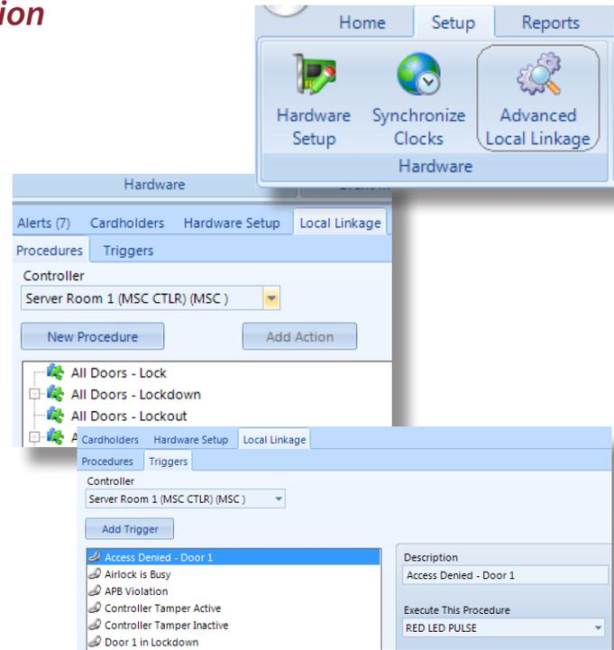
**Advanced Local Linkage** is among the most powerful features provided in Doors.NET when applied to Mercury Powered NXT and authentic Mercury hardware. It is a toolbox for customers to be able to build custom linkage macros to automatically manage or respond to different scenarios without the need for any additional custom software. It is essentially a whiteboard for determining IF (this happens) conditions to execute any THEN (perform these) actions.
